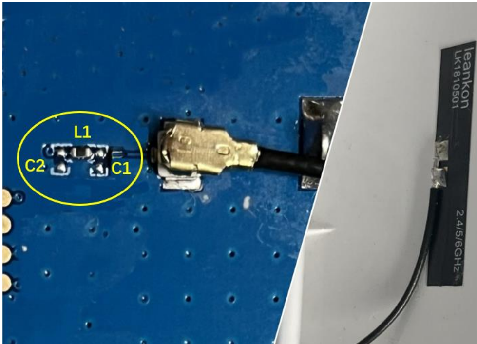
Figure 6.2: The reference PCB layout of matching network
