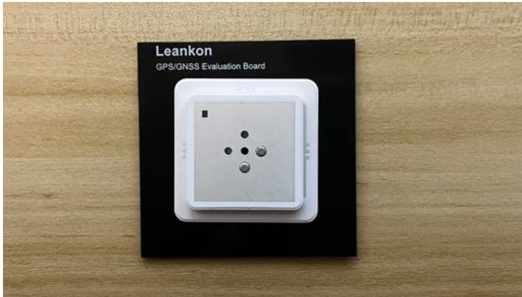
Figure 4.1: The evaluation board (70mm x 70mm x 1mm)
