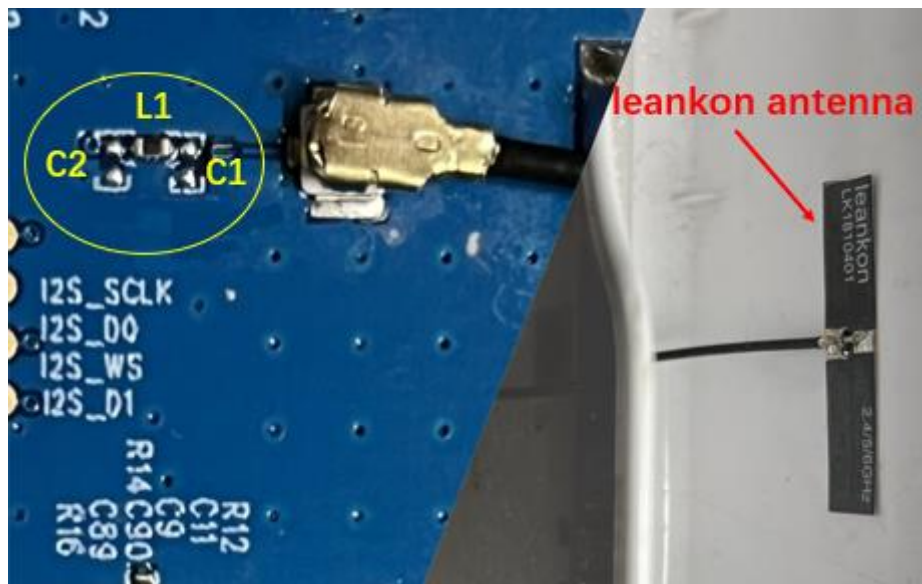
Figure 6.2: The reference PCB layout of matching network
